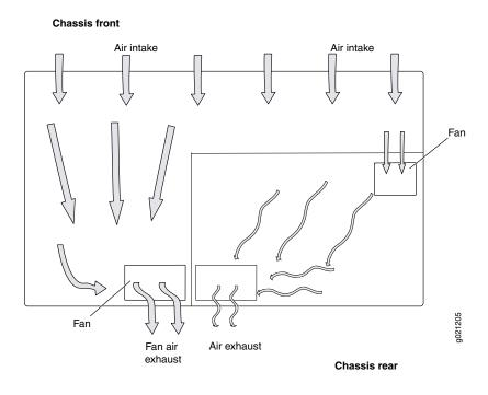
Figure 15: Back-to-Front Airflow Through the EX3300 Switch Chassis
