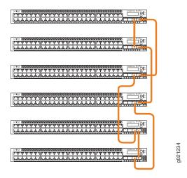
Figure 20 on page 80 and Figure 21 on page 80 show six EX3300 switches mounted on the top rows of adjacent racks and interconnected in a ring topology.
