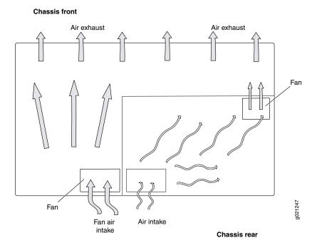
• If you are mounting an EX3300 switch in a rack or cabinet with other equipment, or if you are placing it on the desktop or floor near other equipment, ensure that the exhaust from other equipment does not blow into the intake vents of the chassis.
