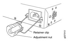
Figure 35: Connecting an AC Power Cord to the AC Power Cord Inlet
