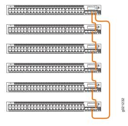
Figure 18: EX3300 Switches Mounted on a Single Rack and Connected in a Ring Topology: Option 2
