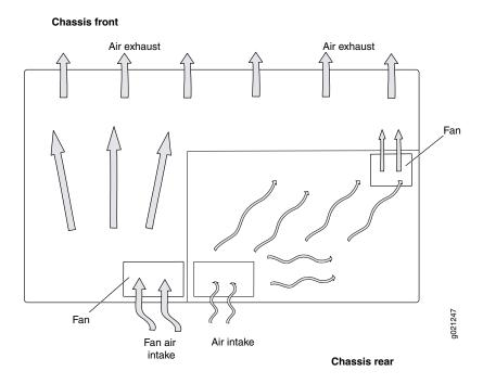
Under normal operating conditions, the fans operate at moderate speeds for minimal noise. Temperature sensors in the chassis monitor the temperature within the chassis. If any fan fails or if the temperature inside the chassis rises above the threshold, the switch raises an alarm and all functioning fans operate at a higher speed than normal. If the temperature inside the chassis rises above the threshold, the switch shuts down automatically.
