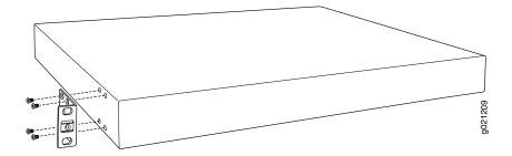
**NOTE:** If you need to mount the switch in a recessed position, use the 2-in.-recess front mount brackets from the separately orderable four-post rack-mount kit.
