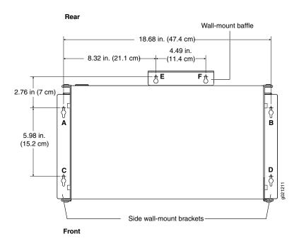
Figure 30: Measurements for Installing Mounting Screws
