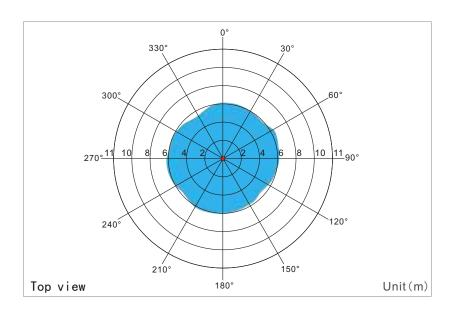
Wall mounted: Angle 130°  $\,$  H 0.8–2m, Front sensing range<15m
