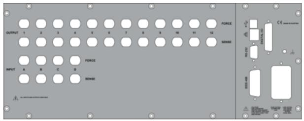
The backside panel has connectors for the matrix inputs and outputs. The switch matrix comes with connectors equipped to the users requirements. These connectors may be of different type. While the relay matrix can always handle high voltage, some connectors may be rated much lower voltage, e.g. BNC/Triaxial connectors are rated 500 V only. It is the user's responsibility only to use voltages which can be handled by the connectors.
