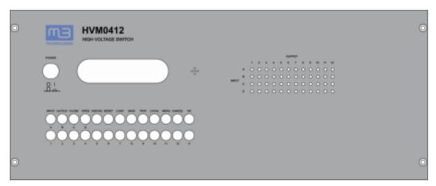
The front panel has several push-buttons, a color graphics display and a led matrix display. The dot matrix display shows the relay status all the time. A green dot indicates a connection between the row and column shown.
