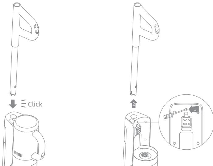
Note: To disassemble, extend a hard object into the hole on the back of the appliance to press contacts and pull the handle upwards at the same time.
