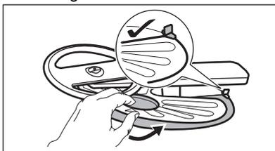
7. Reassemble the filters (B) and (C).
