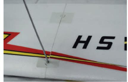
2. Please take out the fuselage and horizontal wing, short wing connecting rod. Insert the short wing connecting rod into the assembly holes from the rudder, then make the connecting rod insert into the left and right horizontal wings. Fix the wings with screw.
