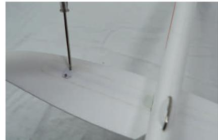
3. Put the assembled main wings to the right position on the top of the fuselage, fix well the wings with screws to the fuselage.
