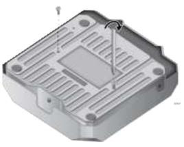
The screw collar provides the proper spacing for the mounting bracket beneath the screw head.
