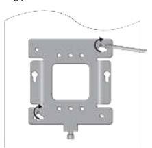
7. To secure the mounting bracket, pre-drill holes through the two bracket mounting holes opposite the key-hole slots.
