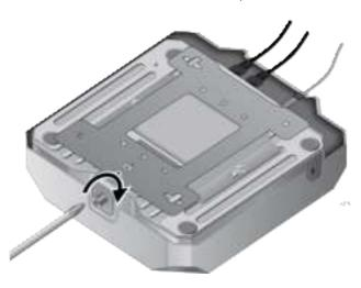
4. Place the Ethernet cable(s) and power cable (if any) along the cable guides inside of the top cover in the cable hiding space.
