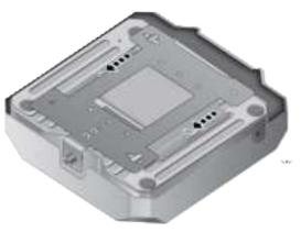
4. Slide the mounting bracket forward and remove it from the access point.
