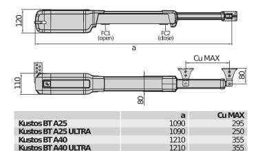
Complete range of electromechanical pistons for residential use, suitable for swing gate leaves up to 4 metres wide and weighing up to 500 kg. Quick and practical installation: the new KUSTOS BT A operators are designed to allow quick and easy installation, thanks to a number of important measures such as the covered worm screw, integrated stops, magnetic limit switches and the magnetic locking pin.
