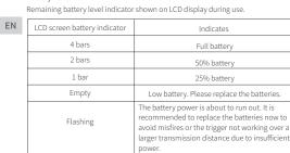
Note: This battery charge indication only please do not refer to this table for NiMH batteries as they are of low voltage
