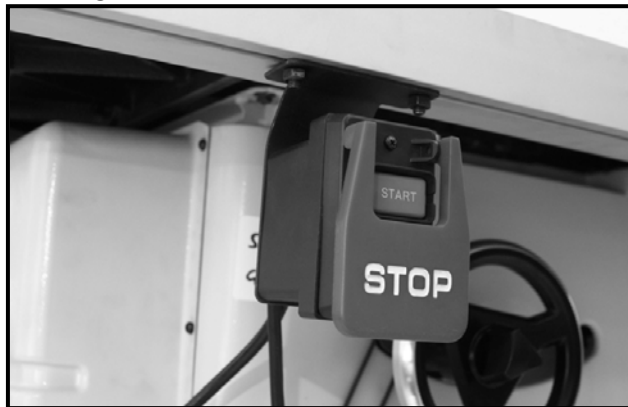
Figure-8 Installing the switch
