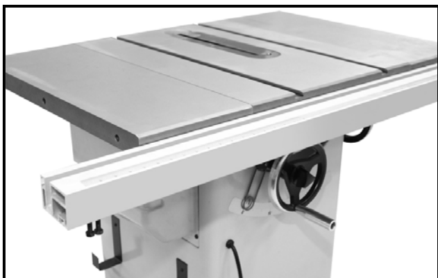
Figure-8 Installing the front fence rail
