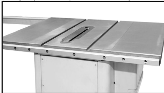
Figure-9 Installing the rear fence rail
