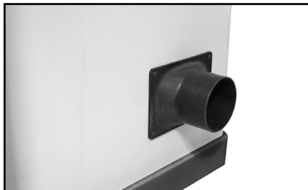
Figure-14 Installing the dust port
