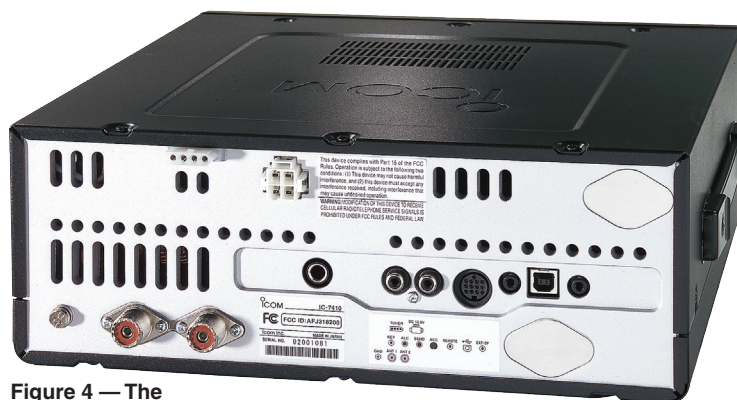
Figure 4 — The uncluttered rear panel of the IC-7410.
