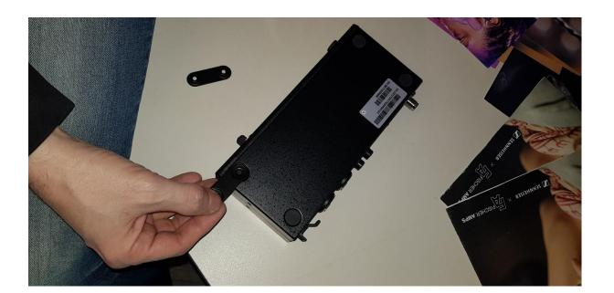
4. The plugs (4) are used to cover the holes in the rack ears for the antennas when they are not in use.
