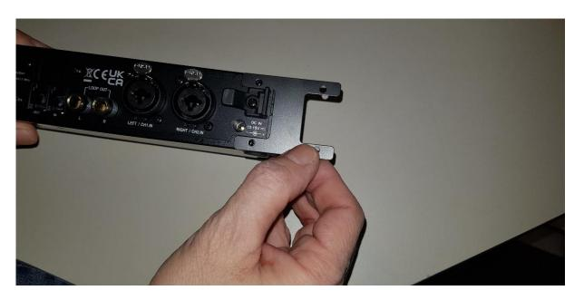
3. The I-connectors (3) go on the inside of the devices. One at the top/front where a screw is mounted to the housing. Please use the screw from the housing.
