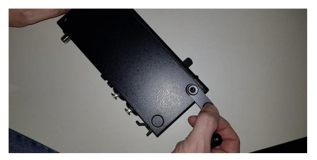
The 2nd I-connection (3) goes on the bottom of the devices, at the front or back. To do this you must remove the rubber foot.
