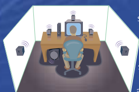
A typical 5.1 system with center channel, front R and L speakers, rear R and L surround speakers, subwoofer and amplifier/controller.
