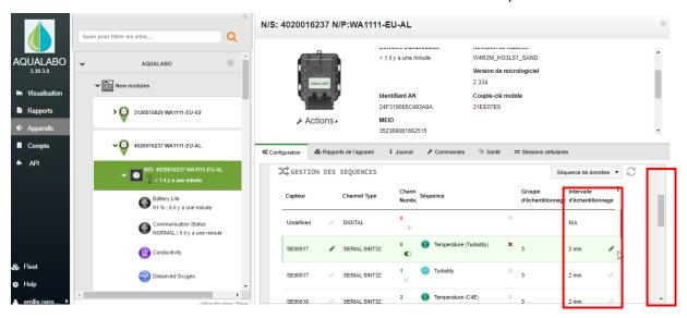
Click it to edit. Indicate the interval desired by the customer. Please note that the time indicated is in seconds! The default frequency is 2 minutes. In the event of a change, it will only be effective at the next transmission. Otherwise, run the magnet over the front panel of the logger to force the transmission.
