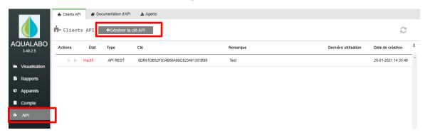
The following window will appear. It is used to generate a secret key that you can enter into your SCADA system (the system uses standard SCADA protocols DNP3 or OPC-UA). You can add a note to it if necessary.
