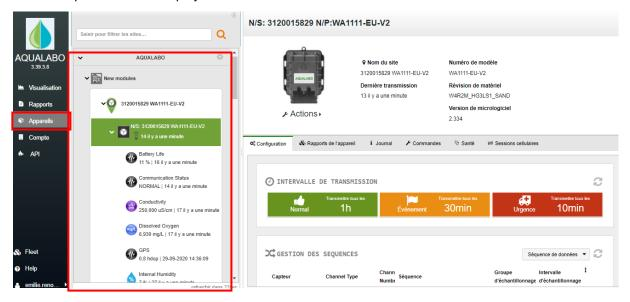
Click on each of the parameters to be configured (as per the sensors connected to the logger). Important: There are at least two parameters for each sensor. Example for pH sensor: pH, Redox, Temperature, i.e. 3 parameters. Configure only the parameters connected to the logger (see parameter table on page 6).
