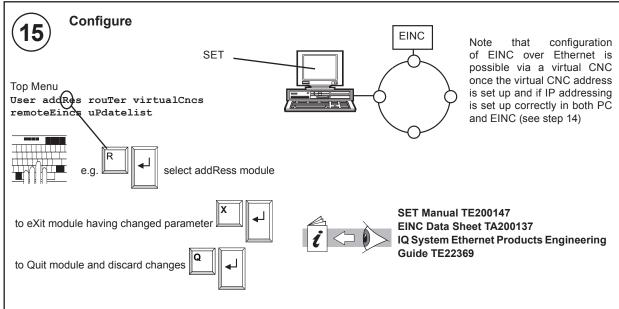
Note that a PIN may be required to make changes in configuration mode. If the PIN has been forgotten the user should contact Technical Support quoting the generator number (User module) and MAC address (address module) whereupon a default PIN will be supplied. This will only work during the same configuration mode session i.e. the utility must not be exited between reading the generator and entering the default PIN. After the PIN is entered a new PIN should be set up and remembered.
