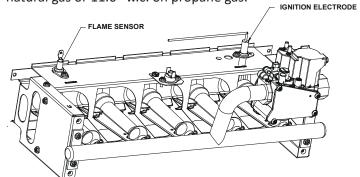
FLAME SENSOR AND IGNITION ELECTRODE LOCATION
