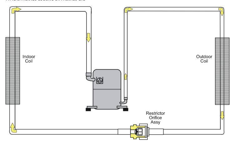
Either a thermostatic expansion valve or restrictor orifice assembly may be used depending on model. Refer to the parts catalog for the model being serviced.
