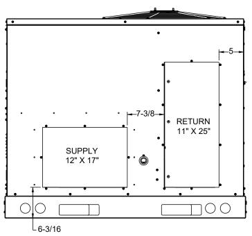
**HORIZONTAL DISCHARGE DUCT CONNECTIONS**
