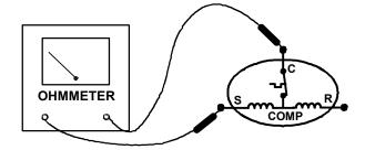
**TESTING COMPRESSOR WINDINGS**
