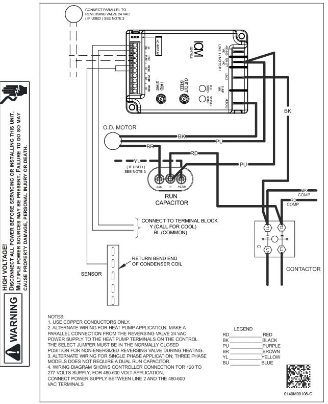
NOTICE: The cut out speed & hard start settings are factory preset. Changing those settings may cause early motor failure.
