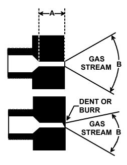
The length of Dimension "A" determines the angle of Gas Stream Defraction, "B".
