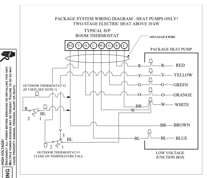
For outdoor temperatures below 0° F with 50% or higher relative humidity, set outdoor thermostat at 0° F
