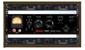
Using the outer set of holes allows you to have 1/2 rack unit of space above and below.
