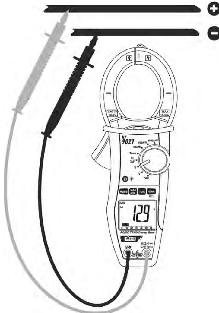
Fig. 4: Taking DC voltage measurements
