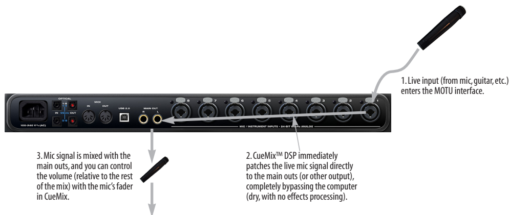
Figure 8-2: This diagram shows the signal flow when using CueMix™ DSP no-latency monitoring. Notice that this method does not allow you to process the live input with plug-ins in your audio software while it is being monitored. You can, however, add effects later — after recording the live input as a disk track. CueMix™ DSP lets you hear what you are recording with no delay and no computer-based effects.
