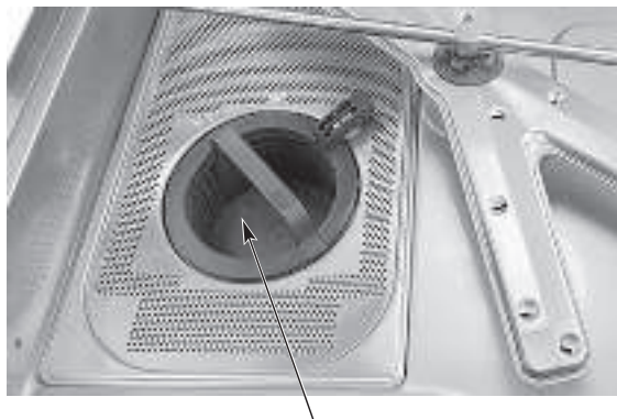
STRAINER BASKET IN UNLOCKED POSITION
