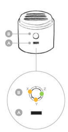
Segment Y to show if the device is powered with cable AND SHOWS WHEN DEVICE IS ON Segment Z to show battery status
