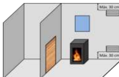
Figure No. 3 - Guideline indications for ventilation grilles
