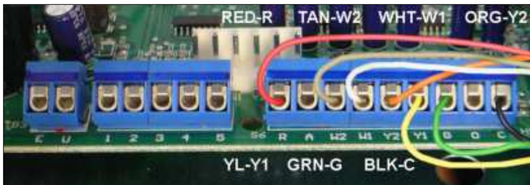
Figure 26: Terminal Connections To TB1 (Sensor Control) On The MTIII Board
