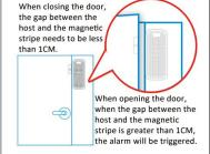
Please note during installation: the triangle mark on the side of the host must be aligned with the mark on the magnetic stripe.
