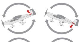
When the plane is rotated up or down (Pitch), elevators should have the correcting actions as illustrated above.
