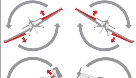
When the plane is rotated left or right (Roll), ailerons should have the correcting actions as illustrated above.
