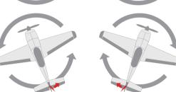
When the plane is rotated to left or right (Yaw), rudders should have the correcting actions as illustrated above.
