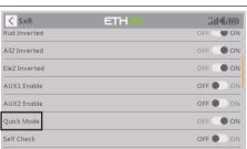
Note: The default mode of SR10+ is Quick Mode. If Quick mode is applied, there is no Knife Edge or (3D) Hover mode.
