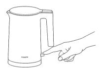
3. Press the on/off button. Then the heating indicator turns on and the kettle starts heating.
