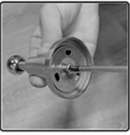
STEP1: Unscrew the base screws
