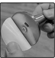
STEP4: Put the adhesive on the gasket
