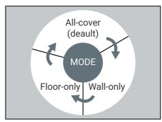
The cleaner will be in All-cover mode after turning it on. As shown above, each press will change the mode.
