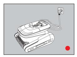
Connect to the power supply - it will then start charging. The LED light will be solid red.
