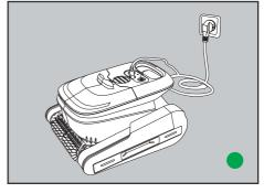
It will be solid green when the device is fully charged, then will turn off automatically in 10 minutes.
