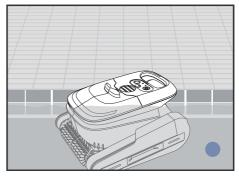
Put the device into the pool, making sure that the water surface is above the top of the machine to enable proper use. The LED light will turn to a solid blue when it starts cleaning the pool.
