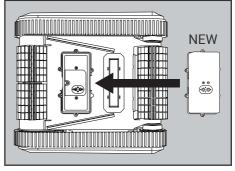
Insert the new battery according to the corresponding contacting positions of used battery.
