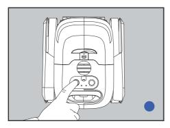
Press the button to turn it on - it will show a flashing blue light, and then it will say: "Welcome to the Seauto pool cleaning robot. I'm ready to work."
