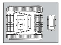
Remove the six screws that used to fix equipment and fetch out the used battery.
