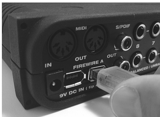
Figure 4-1: Connecting the UltraLite to the computer.
