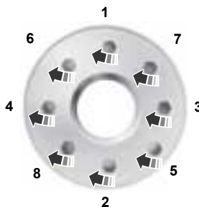
8-lug nut torque sequence
