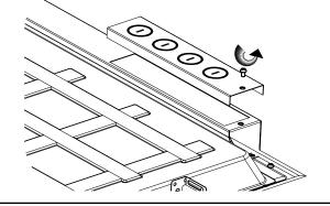
SALE on Nicor Lighting @ www.BulbAmerica.com Connect wiring to j-box with appropriate fittings. Line Voltage 6 Connect wiring as shown. Grey and purple wiring are for 0-10V and 0-10V wiring must be connected in seperate knockouts. dimming systems. Cap off if not used. 0-10V Contro Line Voltage Gnd Wiring Wiring ACL Black ACN White Purple Dim -Gray LED + ● LED -Reattach cover of junction box and secure with screw. 8 Power on fixture and test for proper function.
