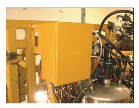
b. Open the air box so that you can see the location of the air control valves.
