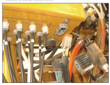
b. Connect the corresponding round and rectangular Deutsch connectors from the AccuBoom cable (P/N 115-0171-579) to the air box connectors.
