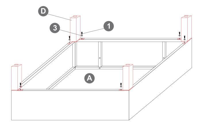
Align holes by placing part C under part A to make installation easier. Tighten the screws 40% to proceed to the next step in the installation.
