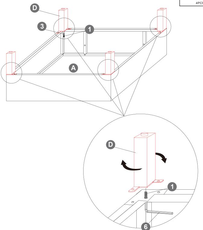
After tightening the screws, tighten the bottom screws
