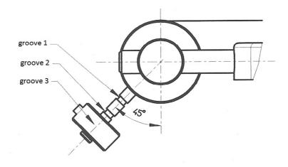
Adjust the anti-skating force by positioning the weight on the appropriate groove of the anti-skating sliding mechanism. Anti-skating downforce should be adjusted in correspondence with the tonearm downforce as follows:
