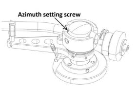
With the aid of a good magnifying glass adjust the needle until it is vertical in the groove (i.e. perpendicular to the record's surface). Ideally this should correspond to the top surface of the cartridge body being parallel to the record surface.
