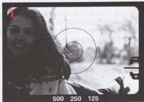
Exposure measurement area
