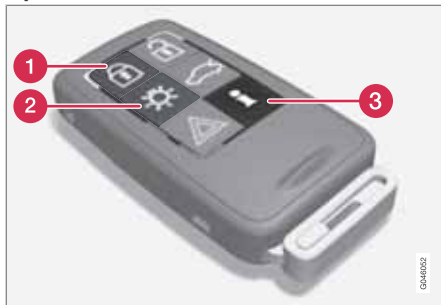
Remote control buttons for remote start.
