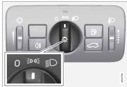
Headlamp control in position for position/parking lamps.
