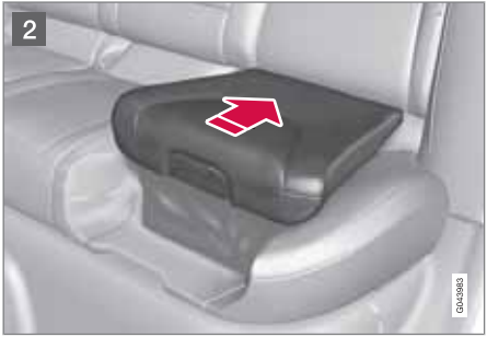
2 Press the booster cushion backwards to lock.
