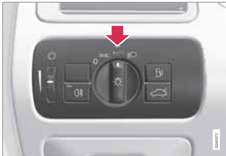
Light switch in position AUTO .
