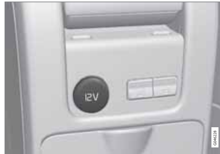
12 V socket in tunnel console, rear seat.
