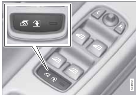
Control panel driver's door.
