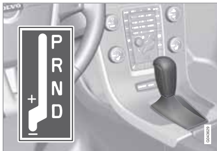
D: Automatic gear positions. +/–: Manual gear positions.
