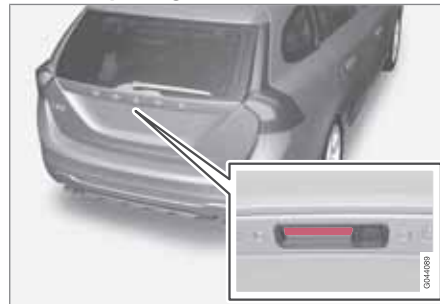
Rubber plate with electrical contact.
