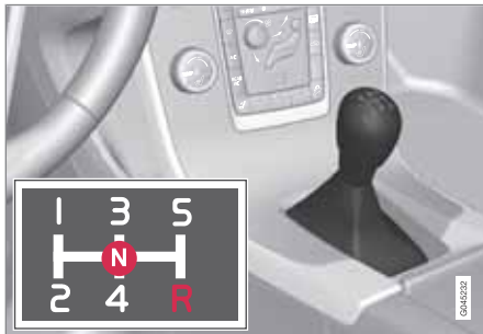
Gearshift pattern 5-speed gearbox.
