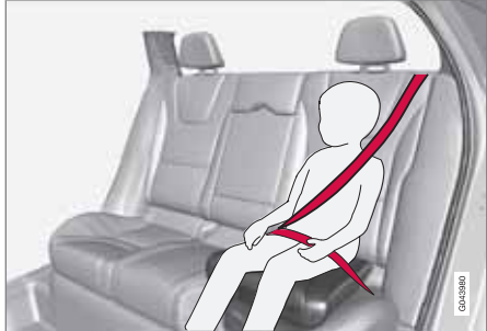
Correct position, the seatbelt should be positioned in on the shoulder.
