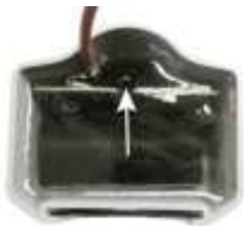
Figure 14: IR LED port ORION Cellular LTE endpoint (bottom up view)
