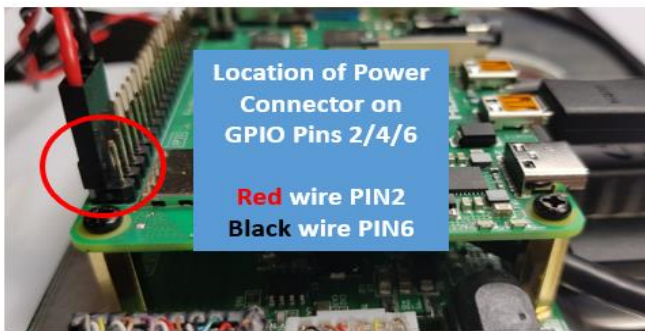
Item #5 – Internal Power Connector (Side view)
