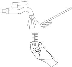
Flush the filter and the adapter.
