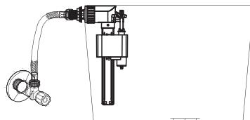
Check the angle valve and the pressure to make sure it matches the requirements.
