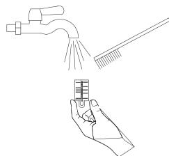
Splaknite filter in adapter.
