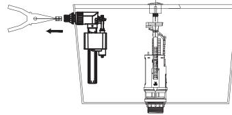
As illustrated, take out the filter from inlet by using pliers or hook.
