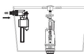
Install clean filter in to inlet and connect the water supply tube as illustrated.
