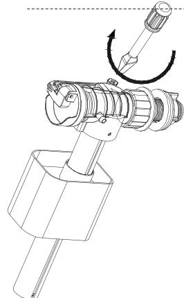
Tighten or release the screw to adjust the water level in a cistern.
