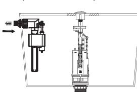
Namestite čisti filter v dovod in ga
