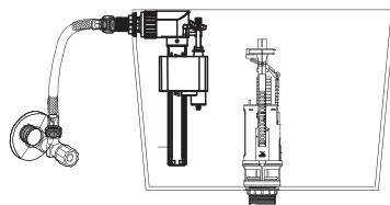
Please turn off the anglevalve before adjusting the height of fill valve.
