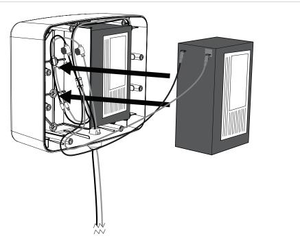
**3.** With the battery(s) in place and connected to the wiring harness, use the four provided screws to secure the Battery Enclosure Kit cover.
