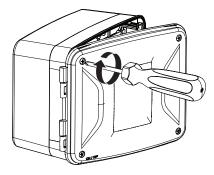
2. The Control Box Cover is then attached to the to the Control Box. The provided Battery Enclosure Kit Cover may be discarded.
