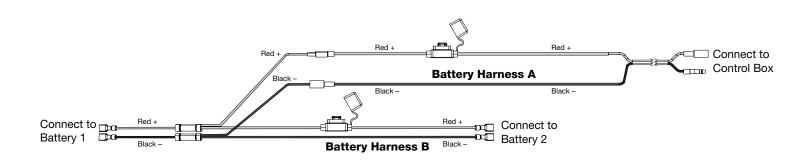
1. Connect the battery harness to the battery as shown: red to positive, black to negative terminals.
