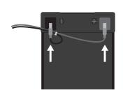
2. Place the first installed battery into the right side of the Battery Enclosure Kit with the terminals facing to the right and towards the top of the Battery Enclosure Kit.
