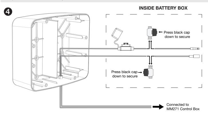
**5.** Splice the two harness sections together using the two provided *IDC Self Stripping Connectors*, ensuring that the new harness will rest within the Battery Enclosure Kit.
