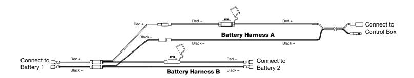
1. Connect the battery harness to the battery as shown - red to positive, black to negative terminals.
