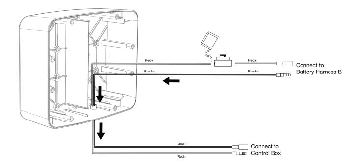
Feed the Control Box end of Battery Harness A through the Strain Relief fitting as displayed above.
