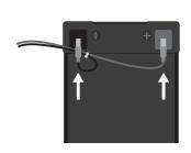
2. Place the first installed battery into the right side of the Battery Enclosure Kit with the terminals facing to the right and towards the top of the Battery Enclosure Kit.
