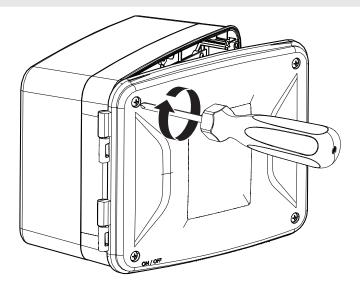
**7.** Align the hinges of the Control Box cover, then close the cover.
