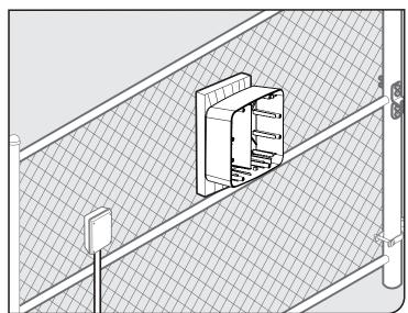
**NOTE:** If the mounting surface is not wood (such as a metal post), you must use a wood panel between the box and the metal post which requires additional hardware (not supplied).
