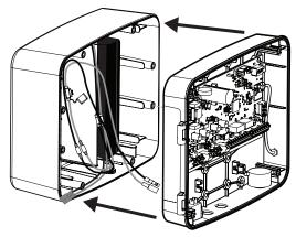
1. Once the Battery Enclosure Kit is mounted, the Control Box will mount onto the Battery Enclosure Kit.
