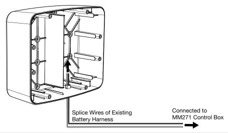
**4.** Feed the spliced end of Battery Harness A (connected to the MM271 Control Box) through the Strain Relief fitting from underneath the Battery Enclosure Kit. The wiring harness will then need to be constructed and sealed inside the Battery Enclosure Kit.
