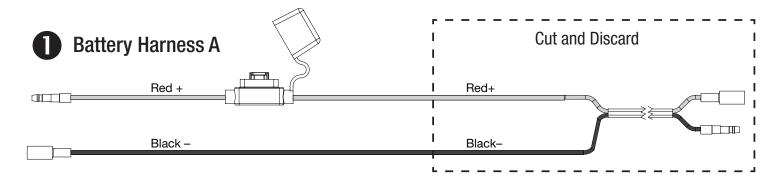
**1.** Cut the section of the provided Battery Harness A.
