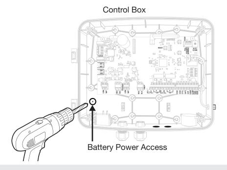
**1.** In order to install the Battery Kit, you'll need to provide wiring access from the Control Box to the Battery Enclosure Kit. With a drill and 1/2" drill bit, drill out the plug designated for Battery Power Access.
