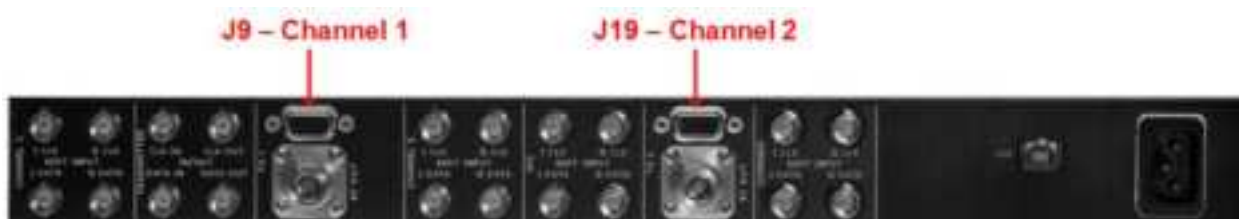
Figure 145: Back Panel with J9 and J19 Labeled
