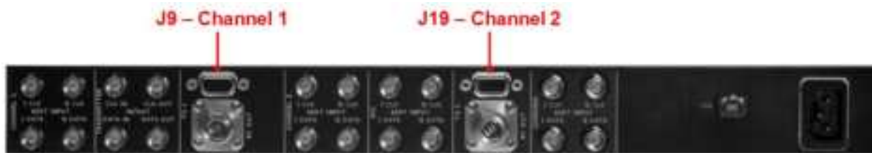
Figure 4: RA Back Panel, J9 and J19 Labeled
