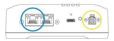
Before connecting PoE to your router, please check specification of your model. Connecting PoE to model that's not supporting PoE can damage your router.
