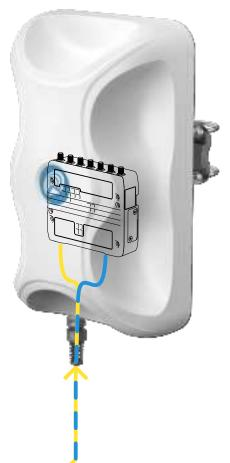
Please note that Semtech XR60 router does NOT support Passive PoE on the ETH port
