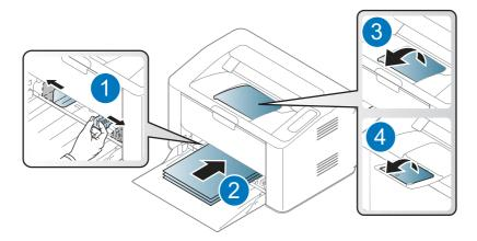
**4.** Squeeze the paper width guide and slide it to the edge of the paper stack without causing it to bend.
