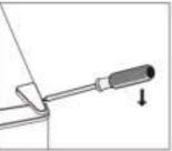
3. Use a Phillips head screwdriver to remove the x3 screws securing the top hinge bracket.
