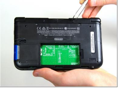
Using tweezers pull out the rubber bumpers that are located at the top of the device on either side
