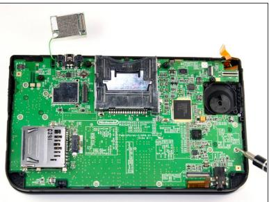
Remove ten 5.5 mm screws that are located around the face of the motherboard.
