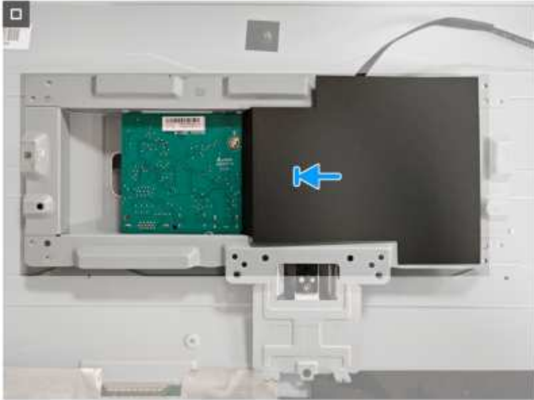
Figure 16. Installing the system board and power board
