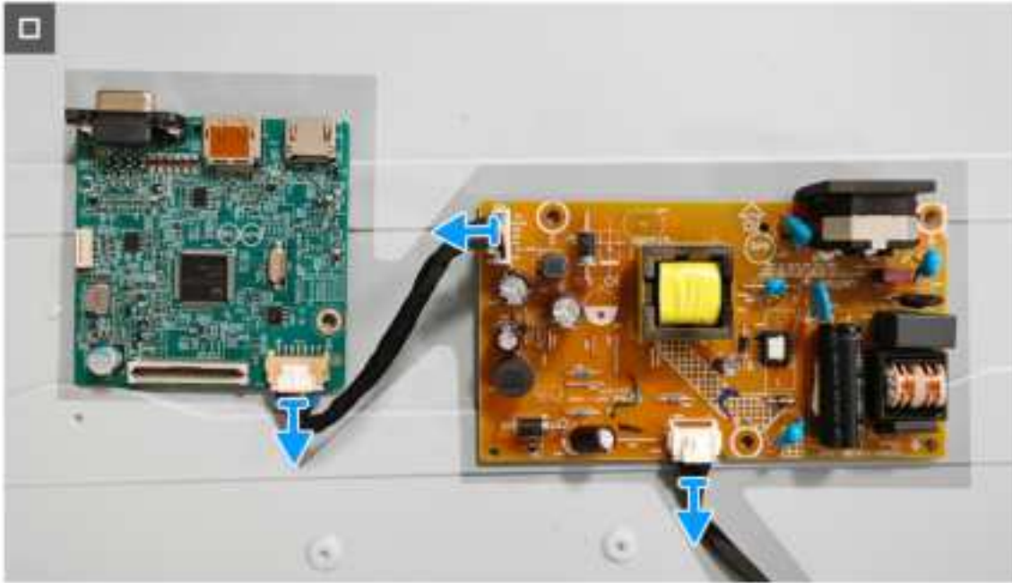
Figure 14. Removing the system board and power board
