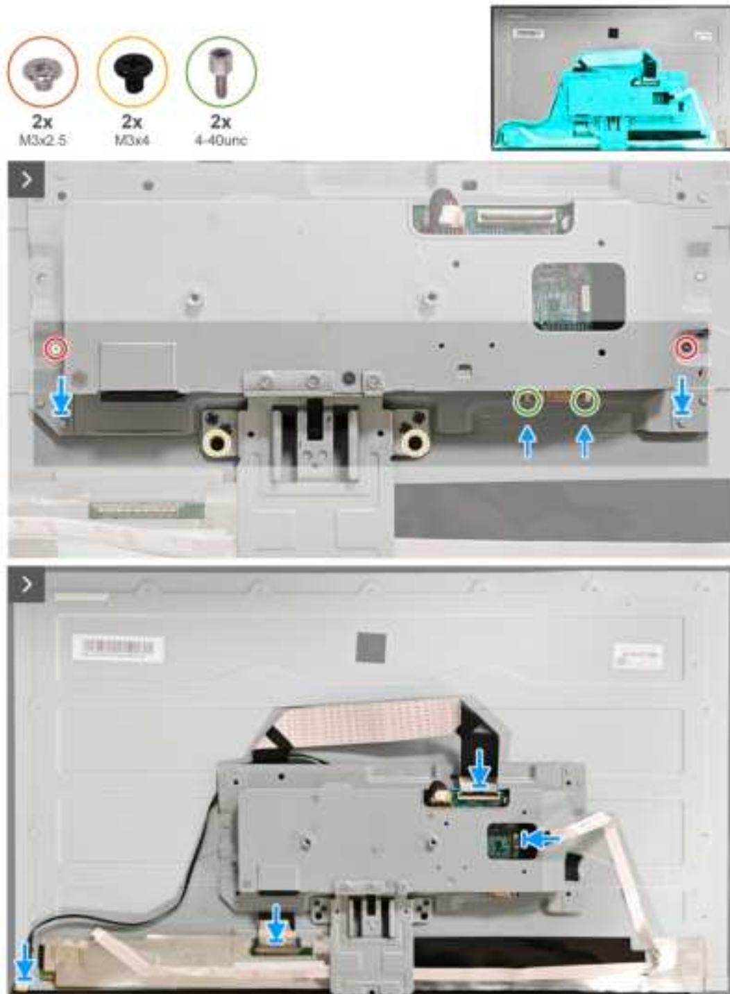
Figure 9. Installing the metal shield
