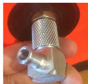
2. Screw on new coupling.
