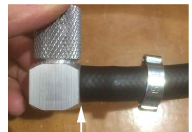
4. Fit hose over hose coupling get hose contact the coupling wall.
