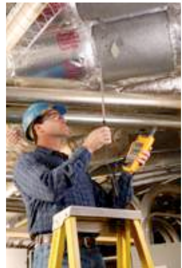
Using the velocity probe to check velocity within a duct.
