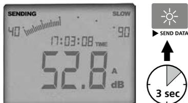
Connect the device to the PC as described under Point 10 and start the program. Press and hold the "SEND DATA" button for 3 seconds to start data transfer. "SENDING" appears on the display. All recorded data are now shown in real time on the PC. Press the "SEND DATA" button again for 3 seconds to stop data transfer.
