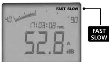
The device features two different measuring intervals. "FAST" time weighting should be set for signals that change quickly. "SLOW" time weighting should be set for continual signals that change slowly. The "FAST" measuring interval is 125 milliseconds while the "SLOW" measuring interval is 1 second. The time weighting can be changed at any time during the measurement by pressing the "FAST/SLOW" button.
