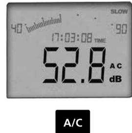
**!** Powerful wind noises (> 10m/s) can affect the measured value. In such cases, you should use the wind deflector supplied with the product.
