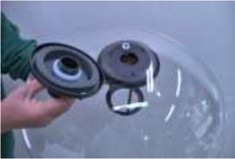
Place Dish over Front Plate & place Backplate hub into threads.
